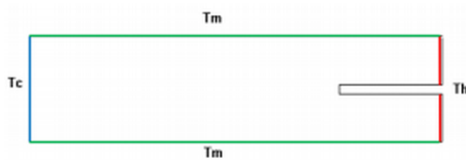
Figure 2 Schematic diagrams of the physical domain, horizontal walls of temperature T_m
